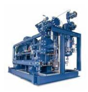
Reliable compressor package with oil-injection. Stepless volume control by hydraulically operated slide valve (slide control). Integrated oil separation, 6 sizes.
