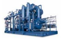
Compressor package with oil-injection. Ideal for gases with light molecular weight, high compression ratio or gases with fluctuating gas composition. Stepless volume control by hydraulically operated slide valves. Design according to API 619 possible.
