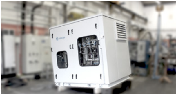
Tilting test to prove safe operation even in wave conditions.
