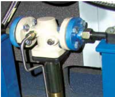
Sealing gas regulator for compressors for exhaust gas compression
