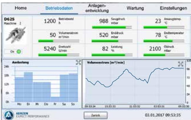
Clicking on an individual machine calls up detailed, real-time data. All the relevant machine data, such as intake and discharge pressure, temperatures, and performance can be reviewed at a glance. For a detailed view, the user can zoom in on the utilisation and the volume flow process.
