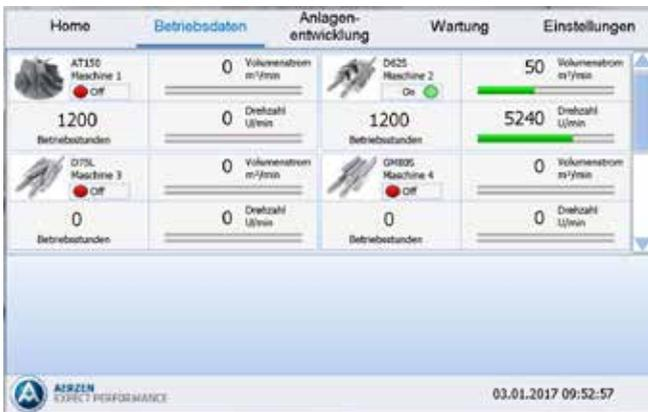
Current data from the entire machine park is displayed in real time. Utilisation values including the current volume flow, the speed of each individual machine, and number of operating hours are presented clearly.
