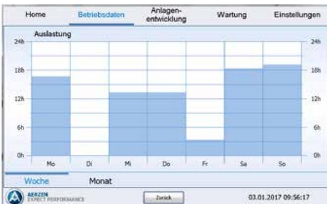
The usage rates of the individual machines are recorded and can be displayed in weekly or monthly view on the AERsmart monitor. The number of operating hours is displayed in the form of a bar chart.
