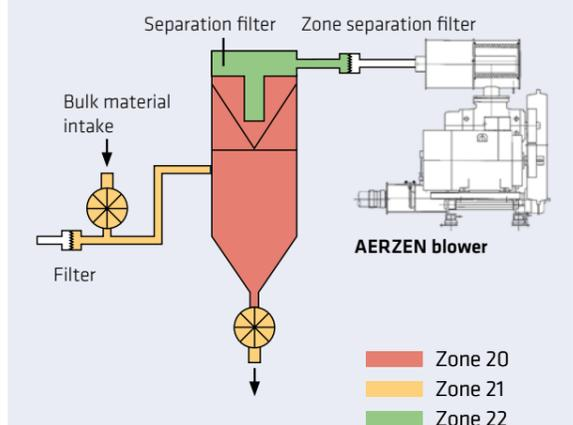
**Explosion Protection in Pneumatic Bulk Material Conveyance.**
