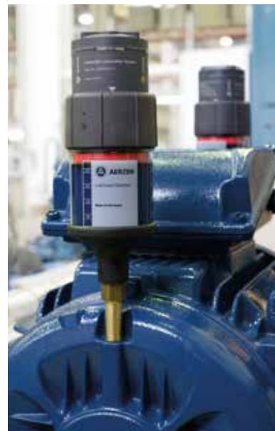
Fixing of the dosing unit with supporting console and screwed connection
