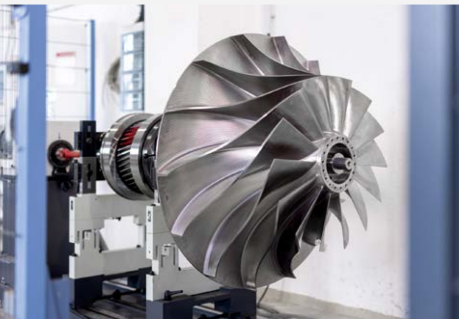
At the GPE balancing station, impellers of up to 1,200 mm in diameter are tested for imbalances at high speed.
