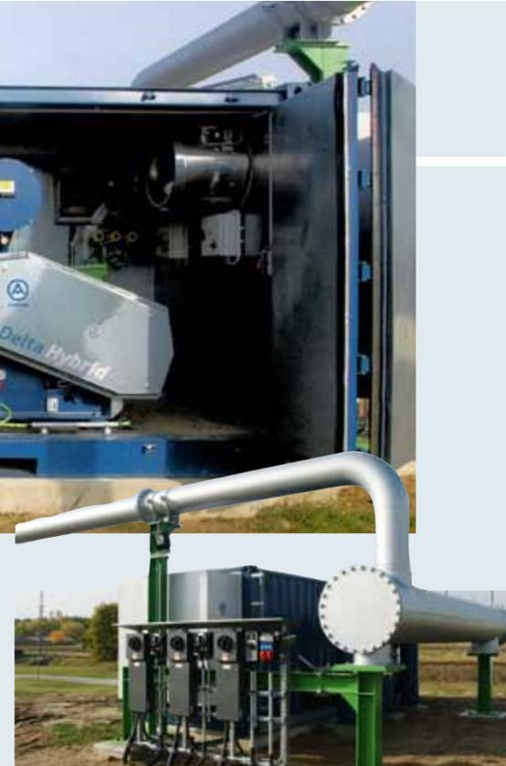
Each rotary lobe compressor can be switched on and off individually from the outside via emergency off switches at the head of the container.
