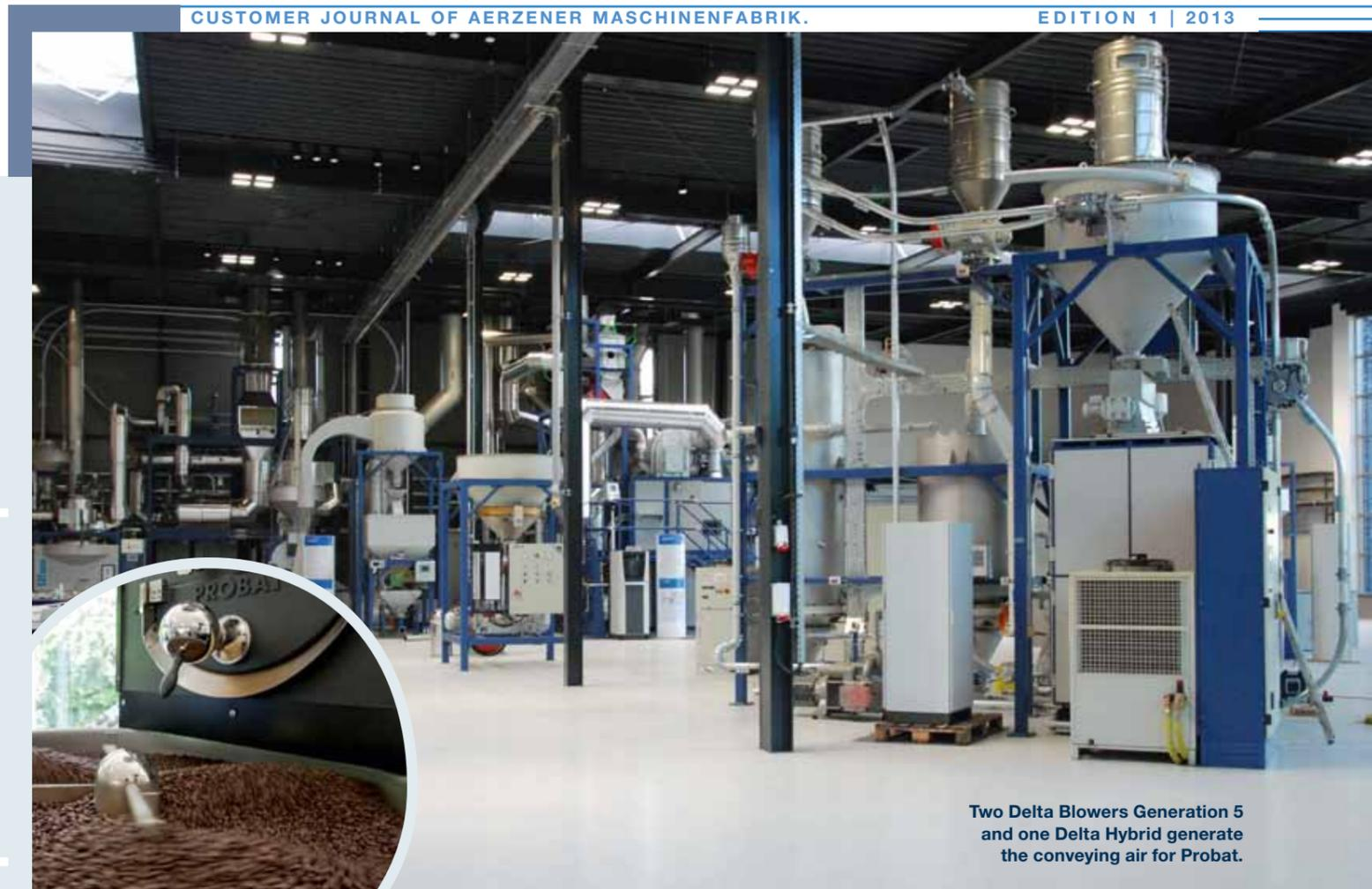
Two Delta Blowers Generation 5 and one Delta Hybrid generate the conveying air for Probat.
