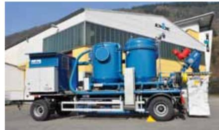
tenance, type GM 35S, generates the negative pressure. It switches off automatically should it encounter a filter surface. The fully automated vacuum cleaning system is operated via an electrical control with SPS.
