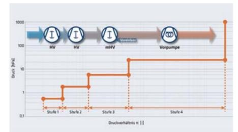
Diagram of a 4-stage pumping set: stages 1 and 2 with HV blower
