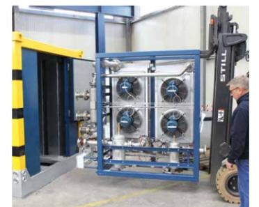
An after-cooling unit constructed like a drawer: the installation as required is carried out by forklift truck and in just a few simple steps.
