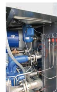
The air-air aftercooler is integrated into the assembly housing.
