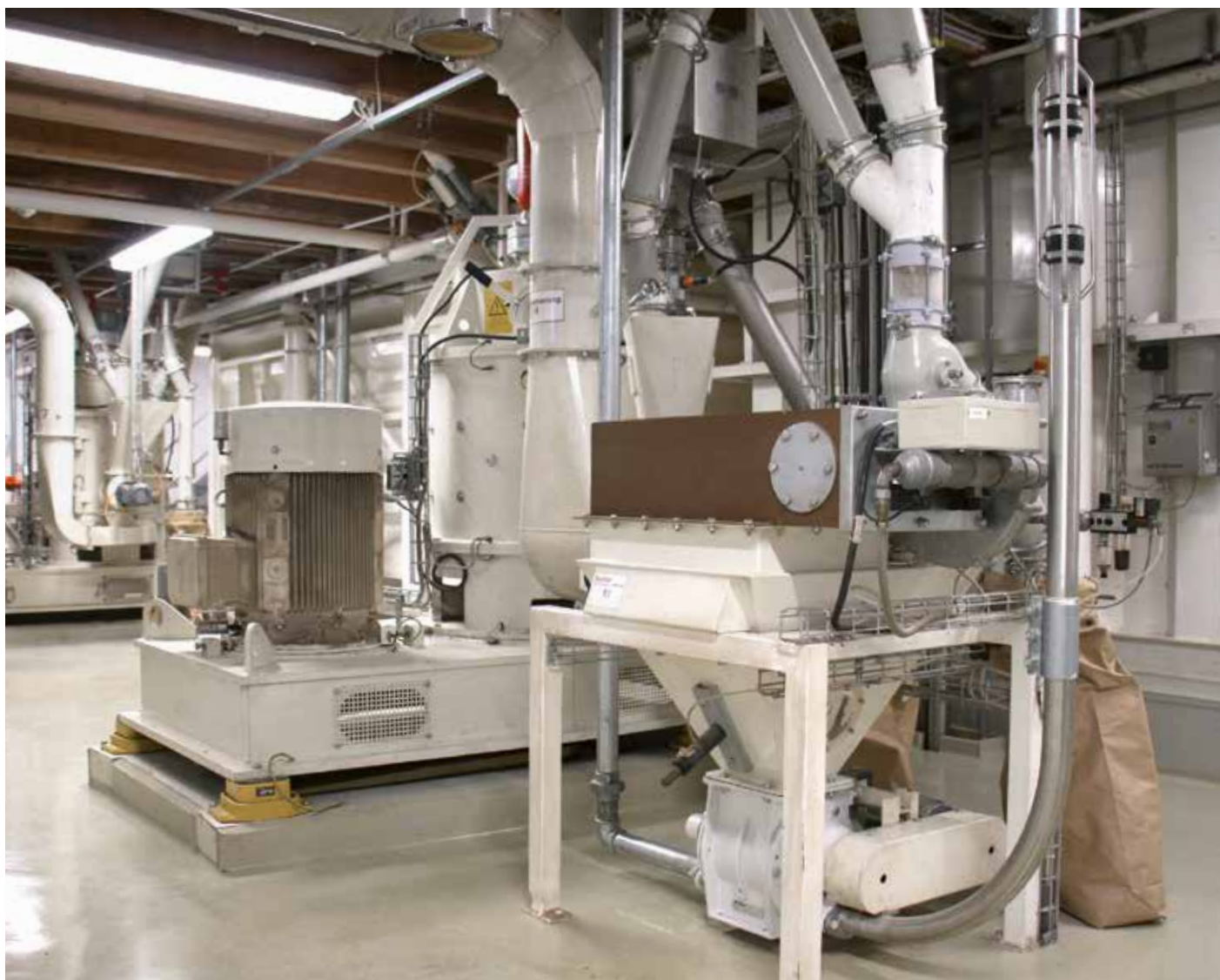
In micronisation, the products are finely ground. Positive displacement blowers made by AERZEN are used for the discharge (silver pipe).
