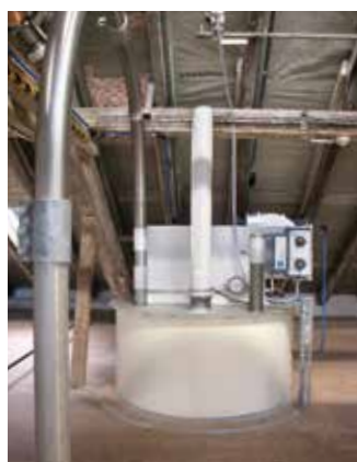
Via the silver pipe, the raw material is transported by AERZEN conveying air from the ground floor up to the fifth floor in the pre-silo for grinding.
