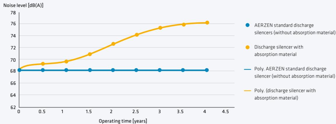
Noise development due to wear of the absorbent in the discharge silencer
