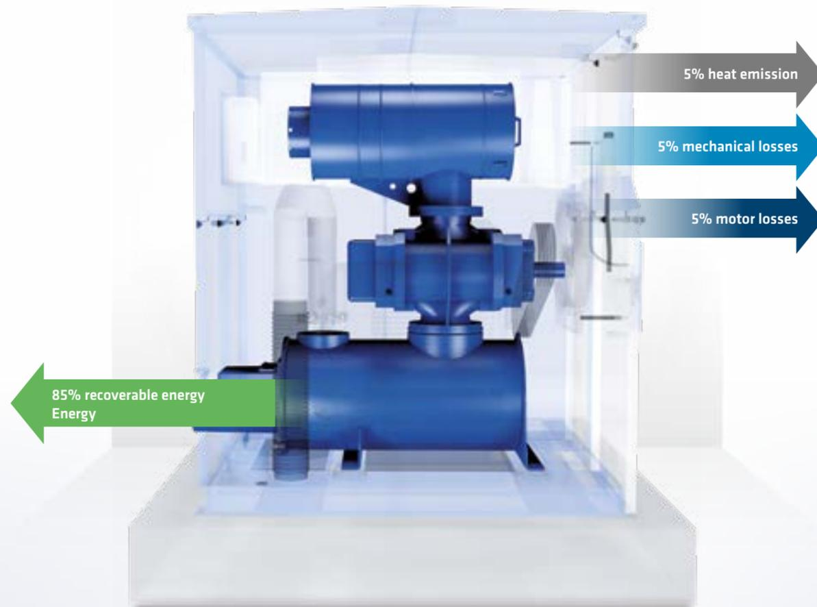
Energy balance of a typical positive displacement blower package
