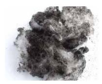
Figure 1: Deposits in bulk material, which collect in silencers with absorption material
