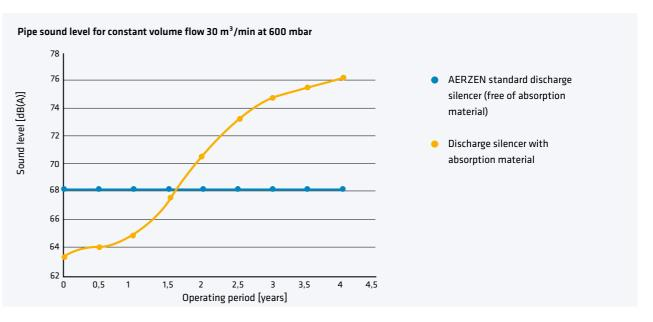
Figure 8: Noise development due to wear of the absorption material in the discharge silencer
