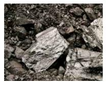
Figure 2: Bulk goods contaminated with oil during the pneumatic conveying process
