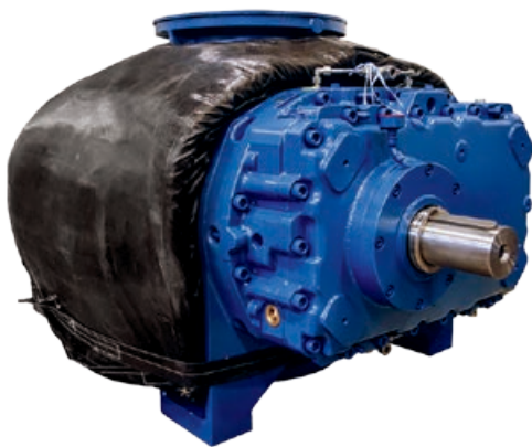
GM 240 S steam blower for ZLD with Ni-Resist D2B steam housing and stainless steel rotors
